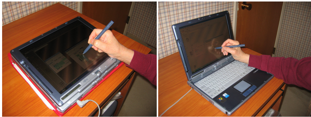
FIGURE 6-1 The Fujitsu Tablet PC used in the experiments, in tablet mode (left) and laptop mode (right).
